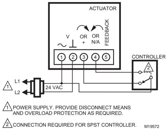
Fig. 10. Wiring for on/off control (floating mode setting).
