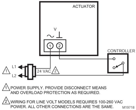
Fig. 9. Wiring for two-position control.
