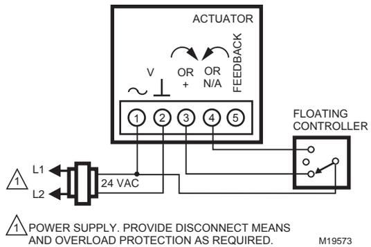
Fig. 11. Wiring for floating control (floating mode setting).
