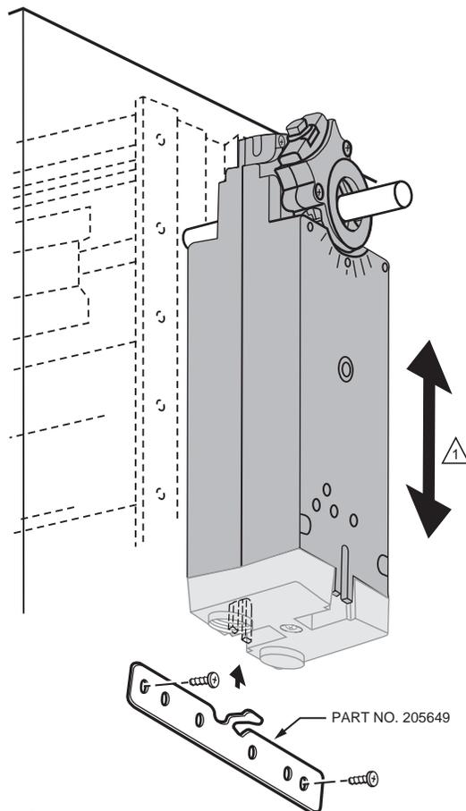
⚠ ENSURE THAT MOUNTING ASSEMBLY PREVENTS ACTUATOR ROTATION AND ALLOWS ACTUATOR TO FLOAT ALONG INDICATED AXIS. WHEN TOO TIGHT, THE RESULTING BINDING CAN DAMAGE THE ACTUATOR OR REDUCE TORQUE OUTPUT.
