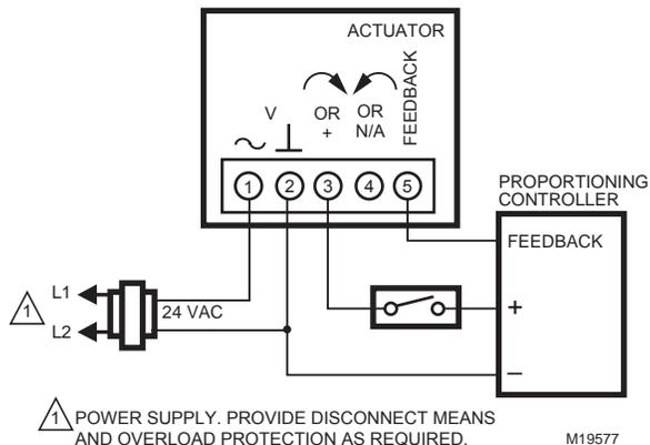
Fig. 15. Override to full close (modulating mode setting).
