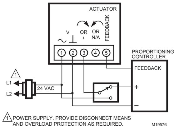
Fig. 14. Override to full open (modulating mode setting).
