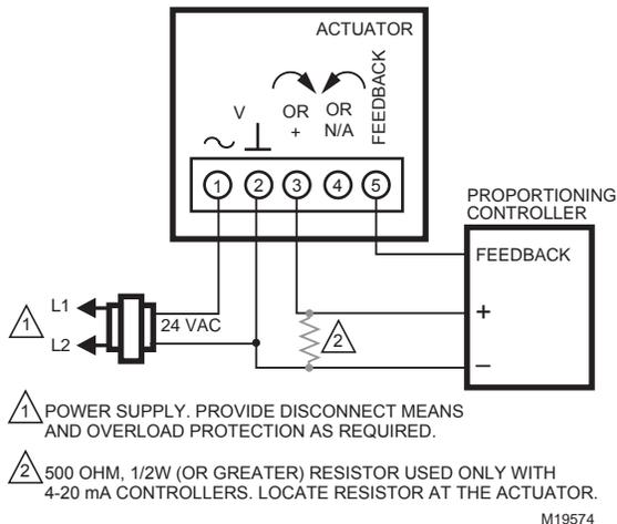
Fig. 12. Wiring for proportioning controllers (modulating mode setting).
